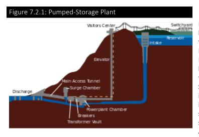
Energy Storage has been in use for a long time, particularly, Pumped Storage-Hydro (PSH). PSH has been used largely for load balancing. Sometimes. ylggus increases or decrease in hydro due to water supply variations. seasonally and daily. And Load varies
